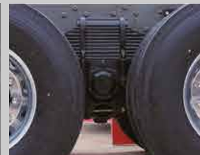
REINFORCED SUSPENSION: Reinforced leaf spring suspension more stiffness and robustness.
