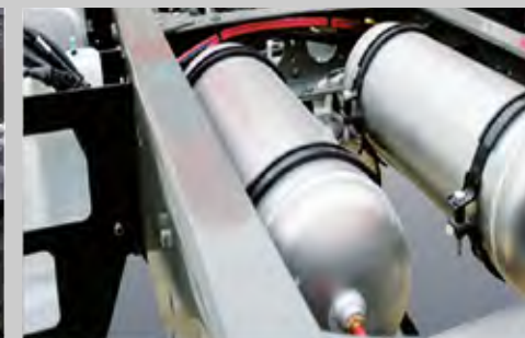
ALUMINUM ALLOY AIR TANK: Anti-corrosion Low weight.
