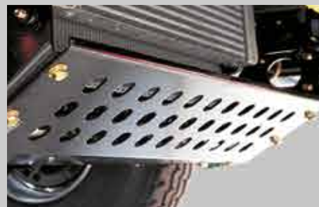
RADIATOR PROTECTOR Withstand stone impact, Better protection
