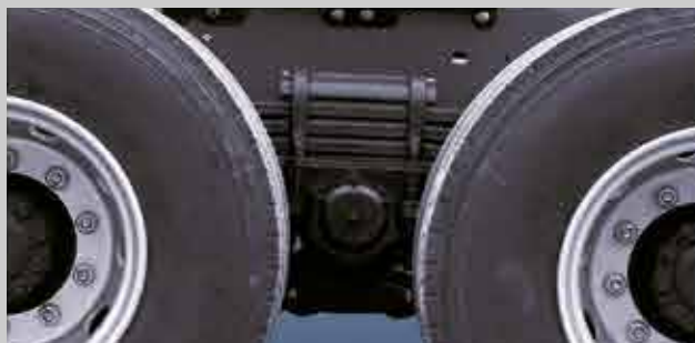
SUSPENSION STRUCTURE WITH FEWER LEAF SPRINGS: High-strength leaf spring, Strong loading capacity, Low weight.
