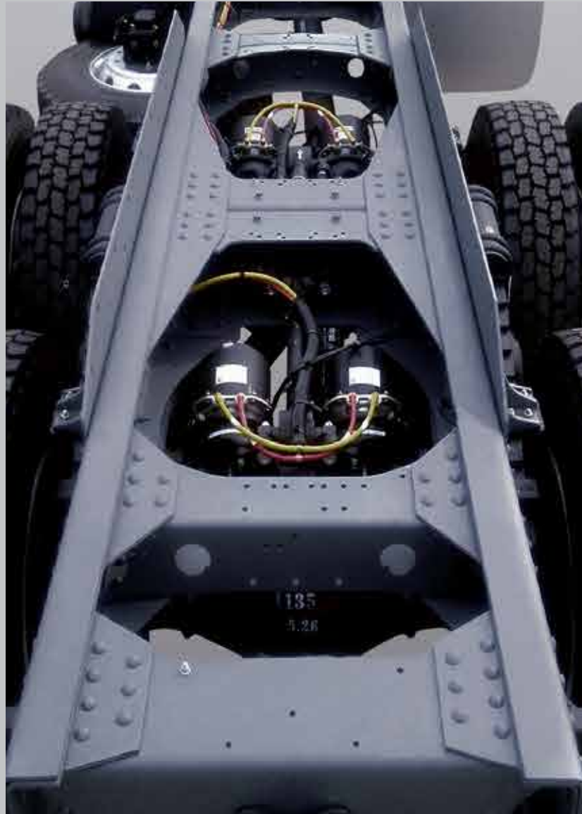
HIGH-STRENGTH STEEL, OPTIMIZED FRAME STRUCTURE; Seamlessly matched mainframe and sub-frame; stronger loading capacity and higher reliability
