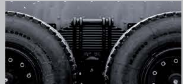
REINFORCED SUSPENSION Reinforced leaf spring suspension more stiffness and robustness with four U-bolt
