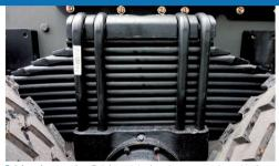
Reinforced suspension Reinforced leaf spring suspension with four U-bolt, more stiffness and robustness
