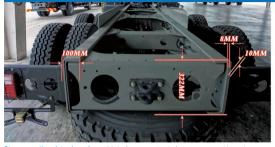
$\begin{tabular}{ll} \textbf{Stamp-one-time-into shape frame} & Main-frame and sub-frame stamped into shape seamless match, the dimension of reinforced frame is $322 \times 100 \times (10+8)$ \\ \end{tabular}$
